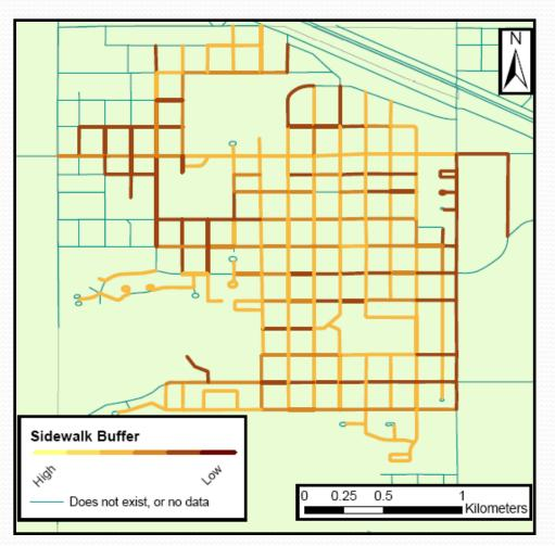
A sidewalk buffer is anything that creates a physical barrier between the sidewalk and the road, for example: a guard rail, or a landscaped strip.
